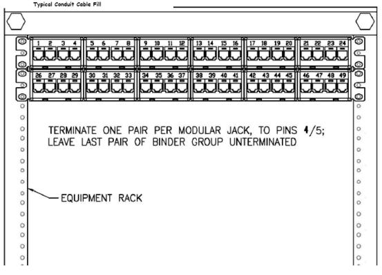
**Backbone Twisted Pair Cable Rack-Mount Termination Example**
